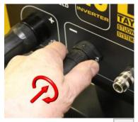
If optional shielding gas is to be used during welding. Attach the bottle supply to the controller via the front panel using a suitable self-sealing push-on socket.
