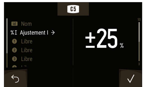
Allows you to adjust the additional current setting (Reg I) from 0 to 50%.
