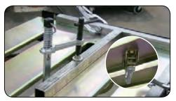
The MagSpring<sup>™</sup> Clamps can be inserted into the 28 mm slots on the Nomad™ Tabletop for hold down clamping. Magnetic V-Pad jaw holds underneath the table to keep the clamp in the up-right, "ready to use" position.
