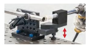
Notch  $25-63.5 \ \text{mm}$  OD pipes or square tubes at any angle, or off-center. Position the two V-Blocks and clamp as needed.
